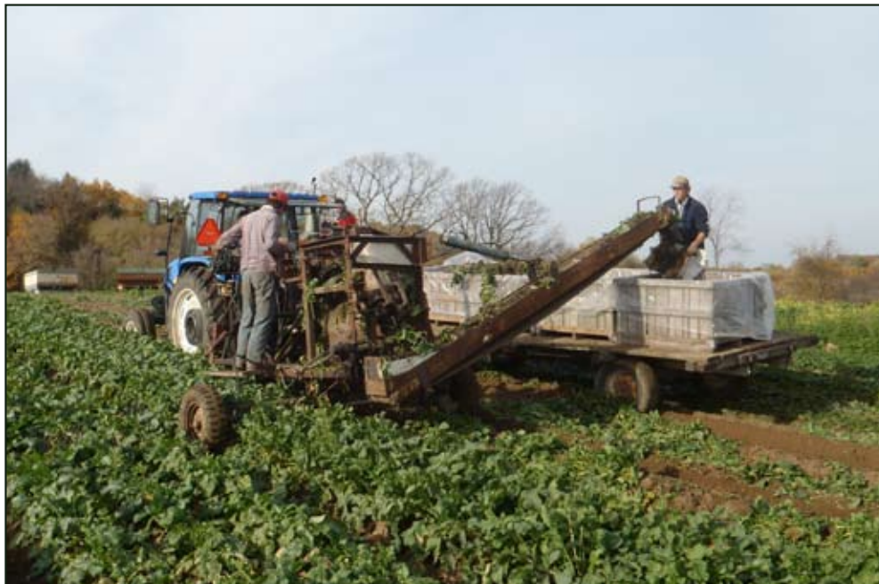
Noah and the gang harvesting winter radishes with the root harvester.
